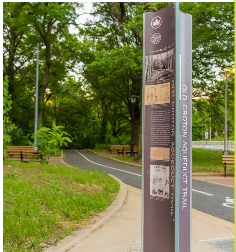
Old Croton Aqueduct Trail by Nancy Owens Studio LLC and Laurel Marx Design is designed for permanence but has some ability to change. Utilizing a landmark sign approach with durable powder-coated graphics on aluminum, the three-part signs can be demounted for replacement with tamper-proof bolts. The signs themselves are placed in more trafficked and highly seen areas to minimize damage.
